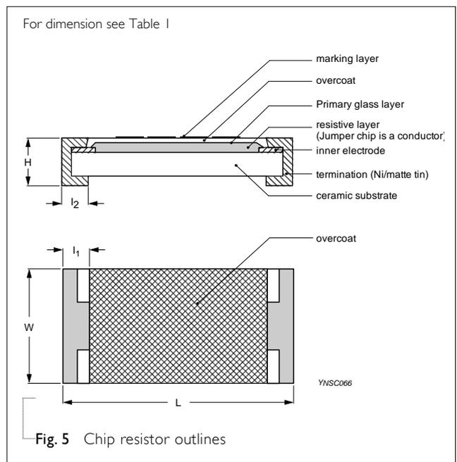
Fig. 5 Chip resistor outlines
