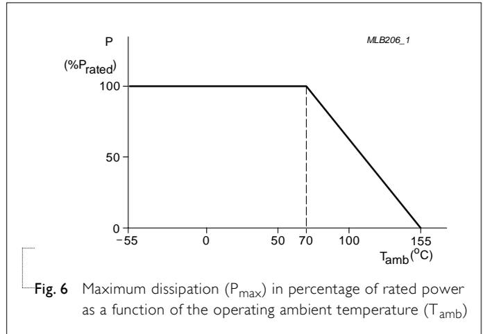
Fig. 6 Maximum dissipation (P<sub>max</sub>) in percentage of rated power as a function of the operating ambient temperature (T<sub>amb</sub>)
