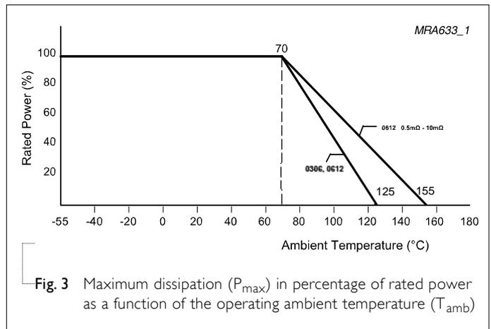
Fig. 3 Maximum dissipation (P<sub>max</sub>) in percentage of rated power as a function of the operating ambient temperature (T<sub>amb</sub>)
