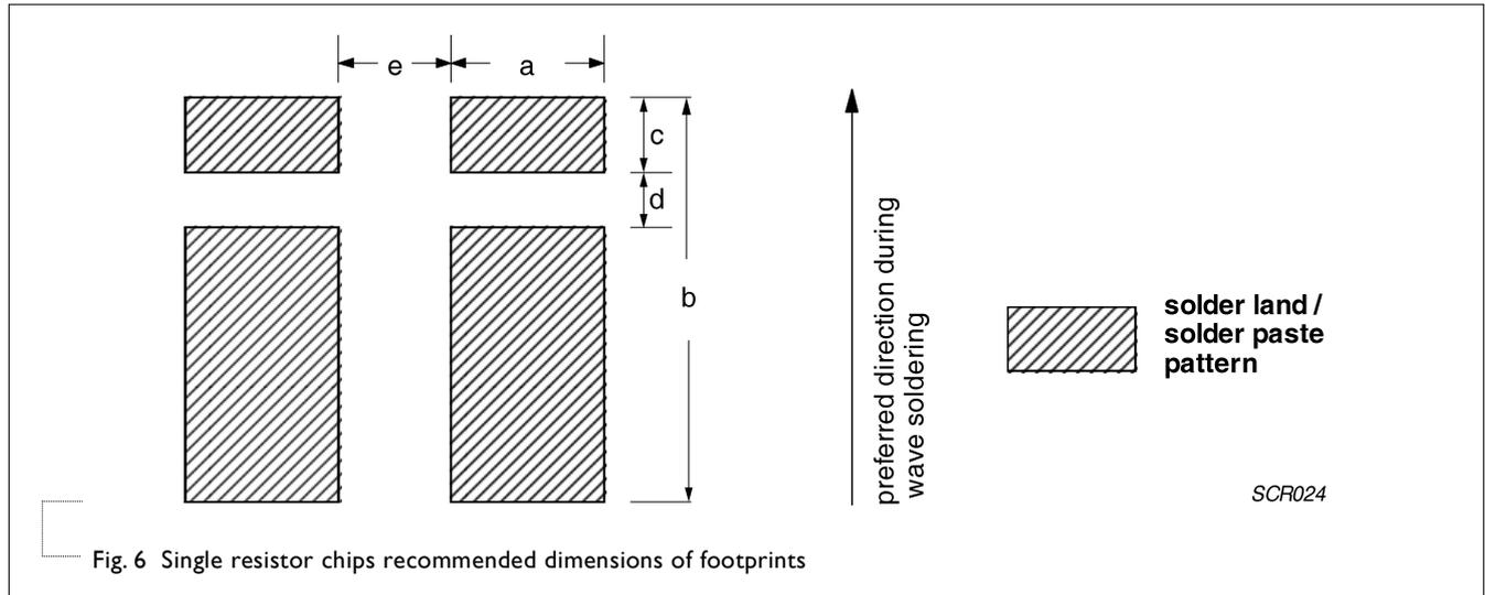
Fig. 6 Single resistor chips recommended dimensions of footprints
