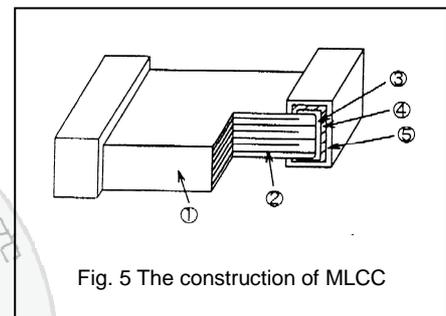
Fig. 5 The construction of MLCC
